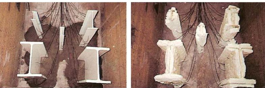
Steel beams treated with intumescent fire protective coating, before and after test fire heat application
